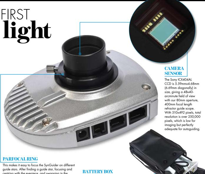
centring with the eyepiece, and swapping in the SynGuider for fine focusing, you put the eyepiece back in with the parfocal ring on its barrel. It's then slid out of the eyepiece holder until the view is focused and then the parfocal ring is locked. Now you'll know that stars in focus with the eyepiece will be in focus in the SynGuider whenever you put it back in the focuser.
